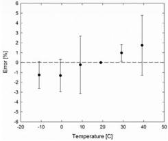
Mean temperature response of eight SQ series quantum sensors (errors bars represent two standard deviations above and below mean).
